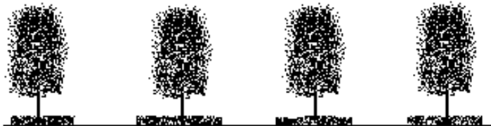
Large trees planted 40' to 50' on center; 3' high evergreen shrubs planted 3' on center
