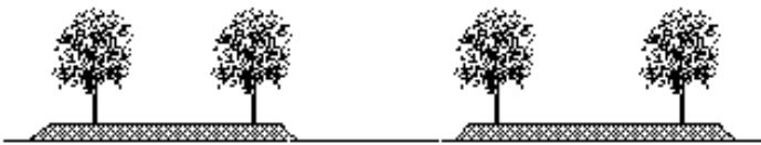
Small trees planted 30' on center on top of 3' high earth berm seeded.
